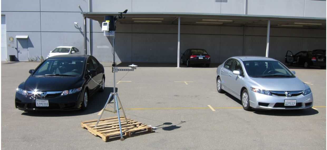
Figure 1. Experimental vehicles parked facing south in Sacramento, CA on July 17, 2010. Tower between vehicles (black car, solar reflectance 0.05, left; silver car, solar reflectance 0.58, right) supports a Davis Instruments Vantage Pro weather station (upper mount) and an Eppley Laboratory Precision Spectral Pyranometer (lower mount).
