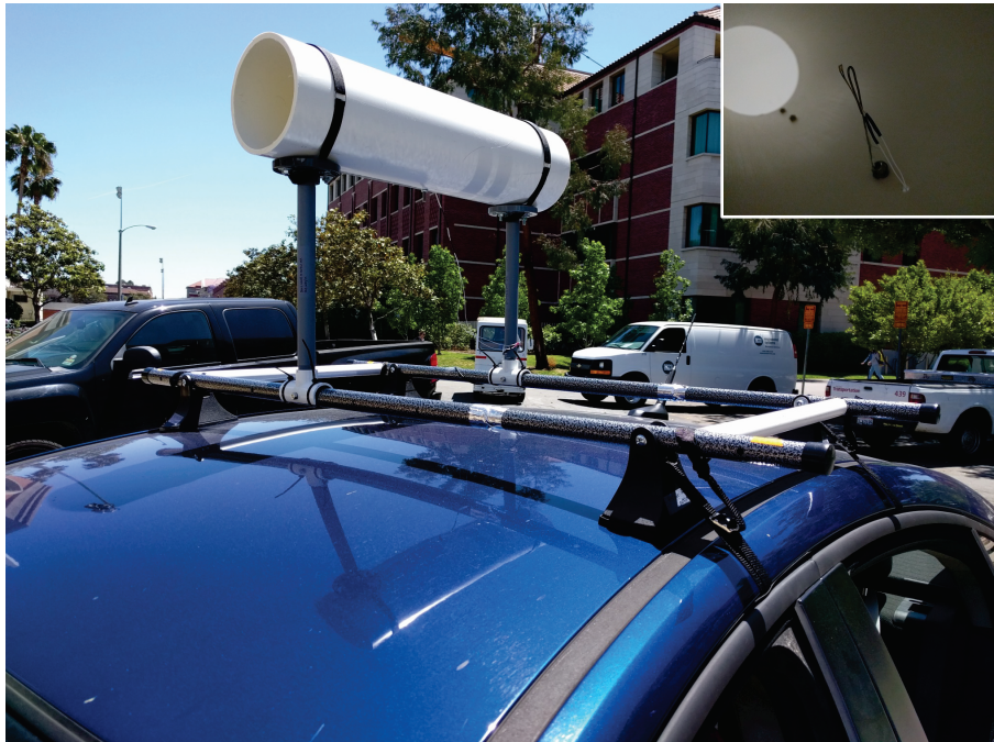
Mobile monitor on quick-install roof mount. Inset at upper right shows high-accuracy temperature sensor centered in white solar shield.
